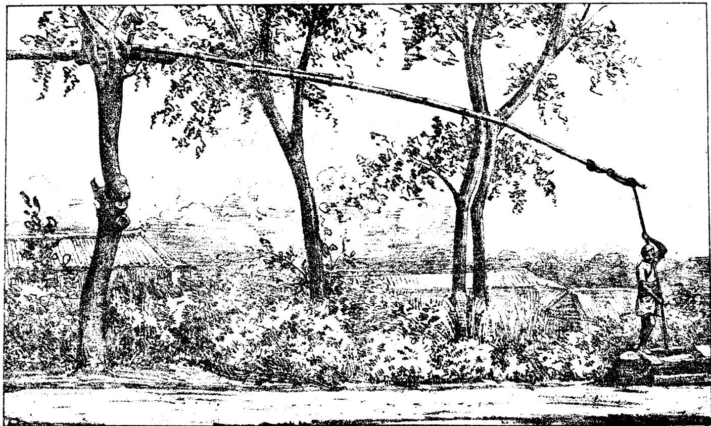
The irrigation lever (latha), pulled down, with the bucket lowered in the well
